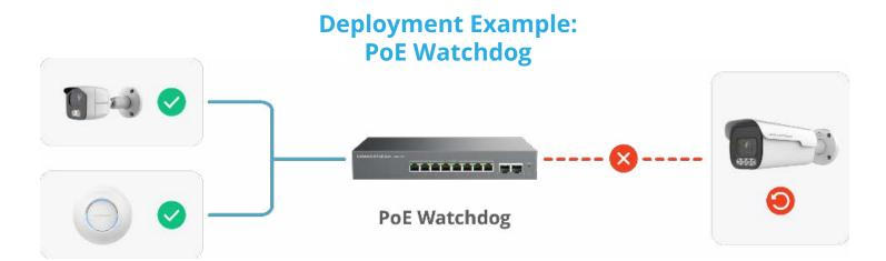
**Anomaly Detection:** The PoE switch continuously monitors the network operation status of connected powered devices (IP cameras, Wi-Fi APs, IP phones, and more).
